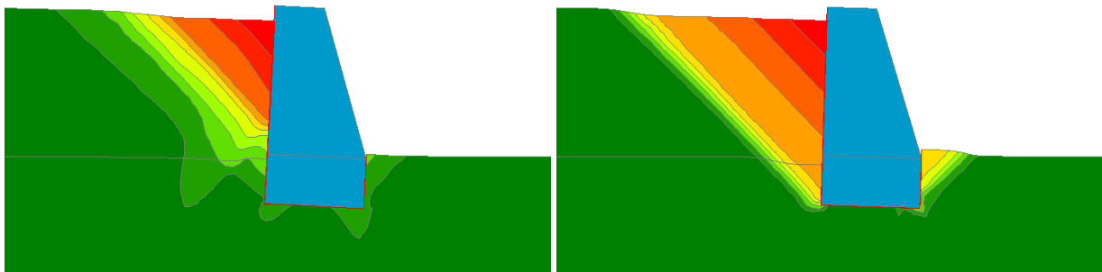
Figure 17: Total displacements |u| with friction (left) or sliding (right) interfaces.
