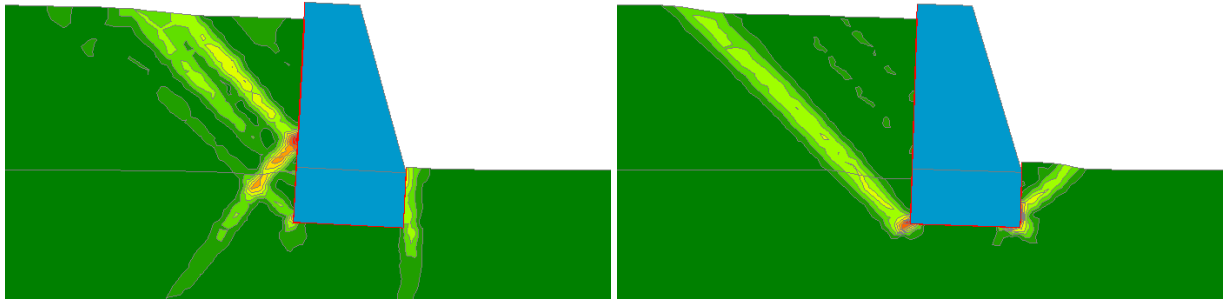
Figure 18: Display of total strains |\varepsilon_1, t| with friction (left) or sliding (right) interfaces.
