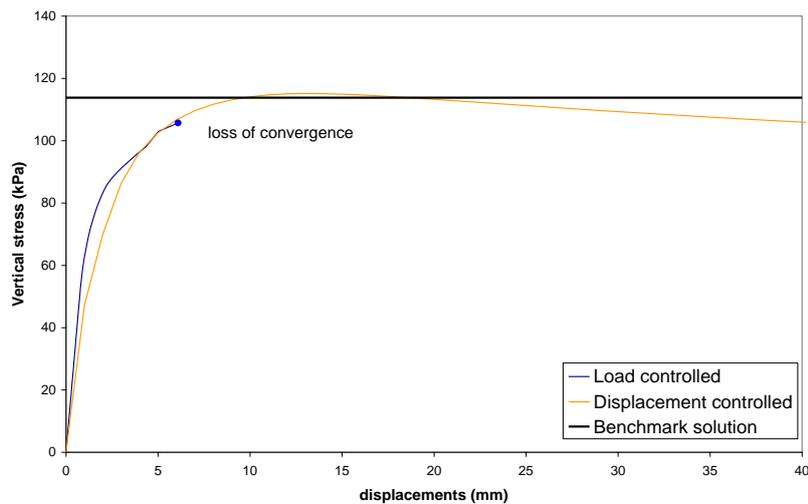
Figure 10: Stress-displacement curve at the centre point of the footing
