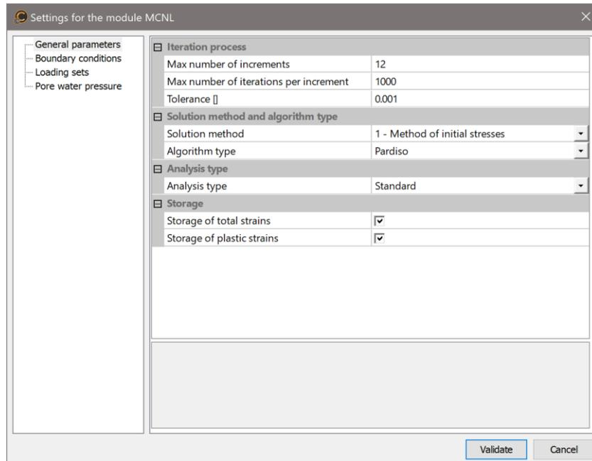
Figure 7: Toolbox for the setting of the calculation parameters
