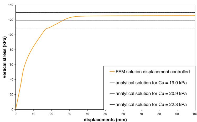
Figure 11: Stress-displacement curve at the centre point of the footing
