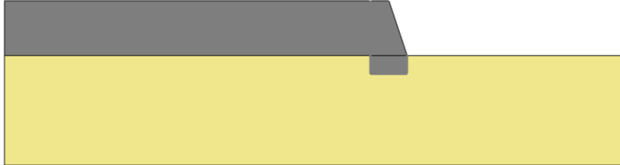
Figure 9: Status of the model when bodies are set inactive at stage #1
