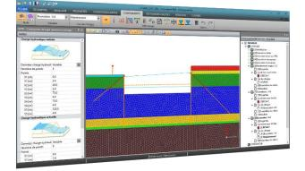
CESAR Graphical User Interface is a fully CAD-oriented work environment. Clear and well-documented toolboxes guide through all the steps of the model creation.
